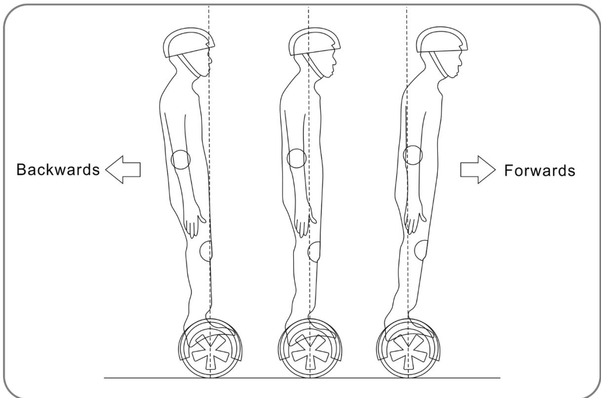
Self-balancing electric scooter has inertial dynamic stabilization system, so it can keep anterior-posterior balance but cannot guarantee the left and right. So when swerved, the scooter need operating slowing, otherwise, you may get injured because of the large centrifugal force.
